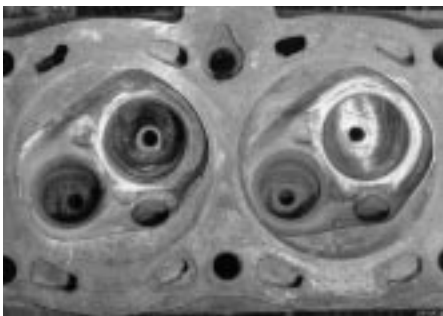
Standard and modified throats and chambers.
