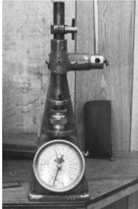
Professional valve spring tester. In drag racing, checking spring poundage is critical.
