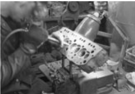
Porting a cylinder head.
