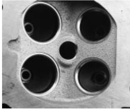
Pent- roof four valve per cylinder chamber.
