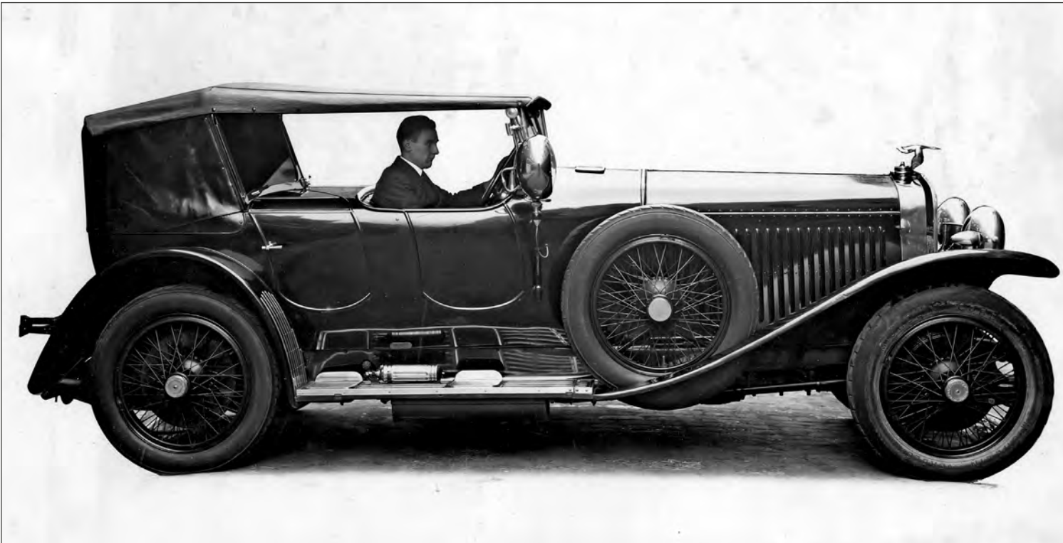
A Saoutchik body was almost always multi-functional. A cover could be stretched between the scaphandrier and the windshield. Note the elegant fender line and the convex door bottoms. Unusually, the sidemounts were not covered. (Nelson V. Thorpe)
