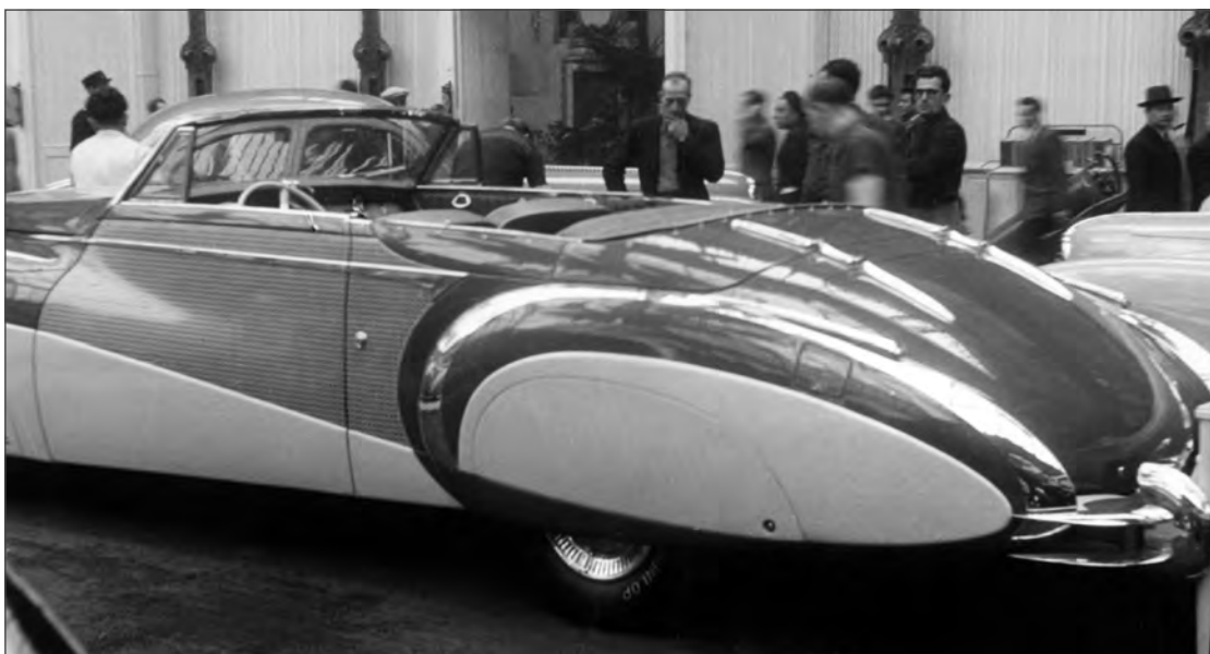
[2/12] The rear end was equally over the top with an immense scallop which completely encased the rear fender. Front and rear bumpers were to a double blade design held together by curved horns. The design was used on Delahaye 175 chassis 815023 and 815044, see following pages. (Zwischengas.com/Automobil Revue)
