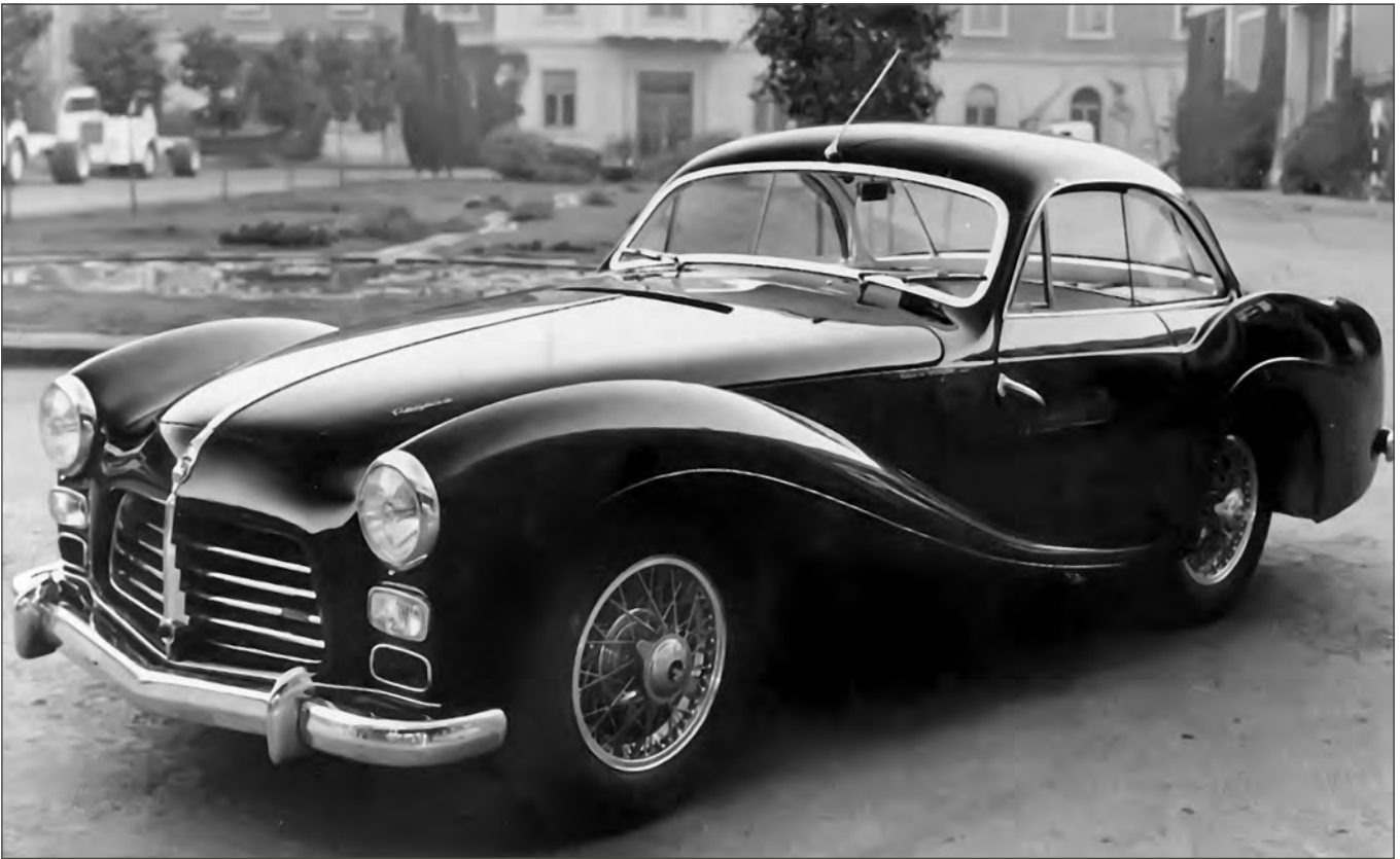
1952 PEGASO Z-102B PROTOTYPE COUPÉ CHASSIS 0117 [1/5] Pegaso Z-102B chassis 0117 was given a prototype coupé body in early 1952. Pierre went for a swoopy non-pontoon design which sat uneasily on the very short 234 cm Pegaso wheelbase. The small kick-up on the rear fender may have been copied from the Pininfarina-designed Series II Nash-Healey coupé and roadster. ( Enrique Coma-Cros )
