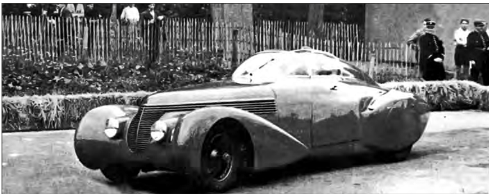
[2/12] At Saint-Cloud, 1946. The body was commissioned by André Dubonnet. It was built on a heavily modified Hispano-Suiza H6C chassis, dating from 1932, which had originally been built to showcase the novel IFS system developed by Dubonnet. The chassis was renumbered 103. (Hervé Pannier)
